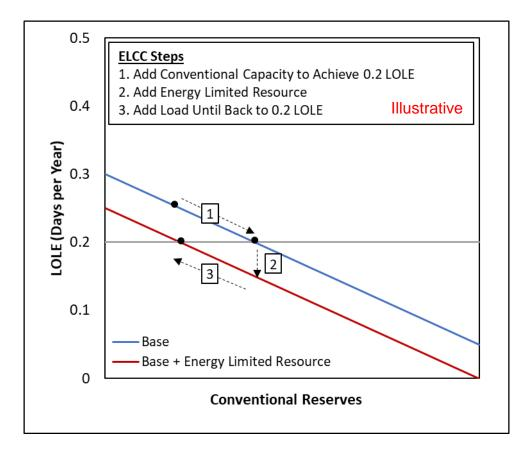
Effective Load Carrying Capability (ELCC) analysis adds load to offset the reliability contribution of the resource type under study. For example, an energy limited resource may be added to the system to improve reliability. This may be offset with load until the reliability target is achieved to quantify the reliability benefit.
