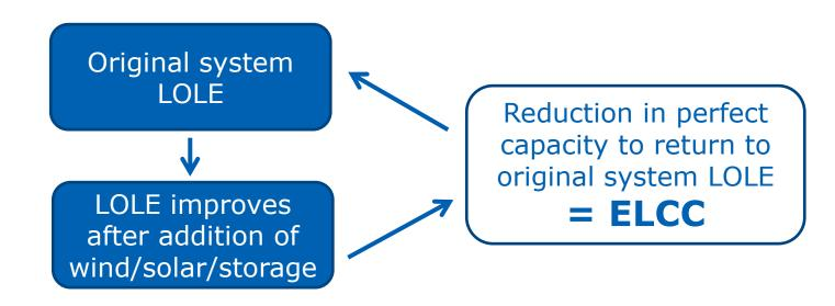
• ELCC is the most rigorous method for calculating qualifying capacity of energy-limited resources (solar, wind, storage, etc.)
